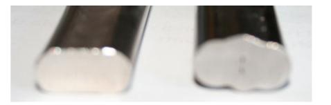
TIG where the two parts jointed are no more visible why a real melting is made and the two partstogether with the adding material generate a new component witout air boubles MIG welding where the two parts are visble and there is the possible oring of air boubles that can originate corrosion phenomens
